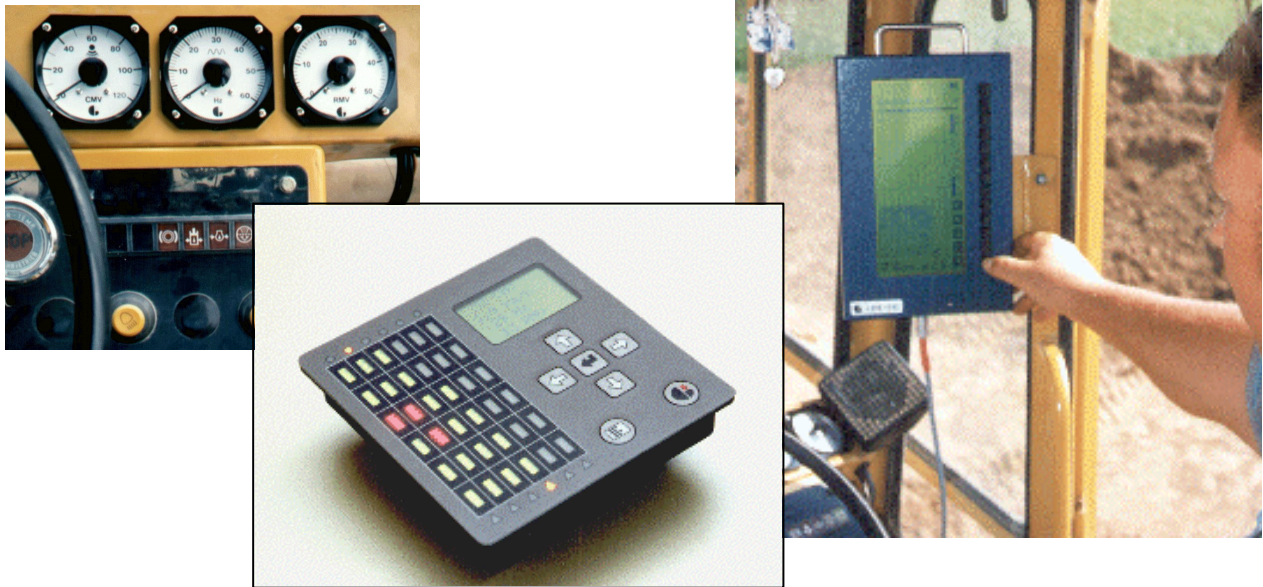
Compactometer dials Compaction Indicator display Documentation system display.
